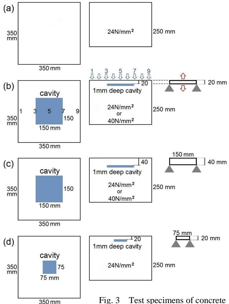
Fig. 3 Test specimens of concrete
