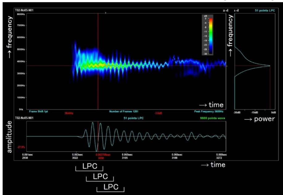
Fig. 1 Spectrogram of abnormal vibrational response of concrete test specimen
